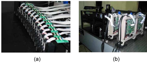
Fig. 1. Pictures of the dynamic holographic stereogram. (a) Curved array of SLMs mounted without upper arms. (b) Whole system with electronic controllers [57]. (J. Hahn, H. Kim, Y. Lim, G. Park, and B. Lee, "Wide viewing angle dynamic holographic stereogram with a curved array of spatial light modulators," Opt. Express , 16, 12372-12386 (2008), © 2008 OSA. Reprinted with permission.)
