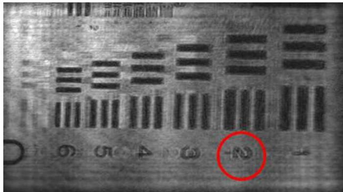
Fig. 2. Numerical reconstruction of the holograms for an object tilted with an angle of 55 degrees as acquired by the CCD ([Movie\\_1](#)).
