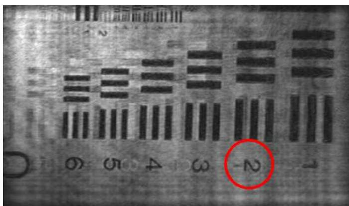
Fig. 3. Numerical reconstruction of the holograms for an object tilted with an angle of 55 degrees after the quadratic deformation.
