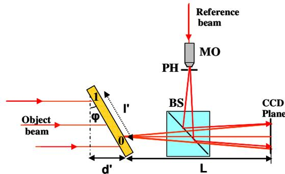
Fig. 1. Experimental set-up: BS, beam splitter; MO, microscope objectives; PH, pinhole.
