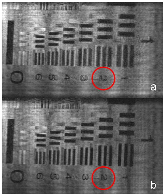
Fig. 4. Numerical reconstruction of the holograms for an object tilted with an angle of 75 degrees as acquired by the CCD (a) and after the quadratic deformation (b).
