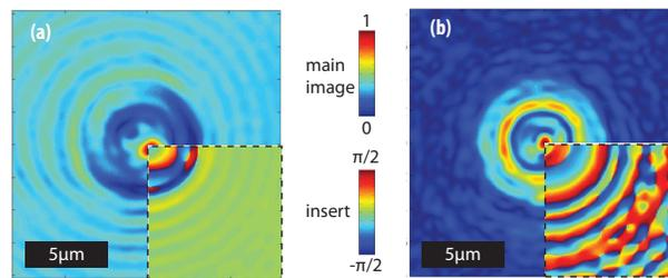
**Fig. 1:** Complex field (main: amplitude part, insert: phase part) of RI-unmatched glass sphere at  $15^\circ$  of sample tilt. Image (a) shows the distorted measured complex field, while the aberration compensated complex field is depicted in image (b). Background and diffraction patterns are successfully removed and the expected symmetric object is only visible in image (b).
