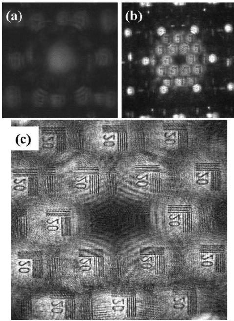
Fig. 4. (a) Reconstructed intensity map at a distance  $Z_T/3$  from the LN-ASF. (b) Reconstructed in-focus virtual images and out of focus real images for each diffracted order, for  $d=d_1+d_2$  (on the target plane). (c) Magnified view of the in-focus multi-images [central part of (b)].
