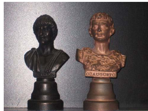
Fig. 11 The two small bronzes which were used for testing. One of them (Augustus) was sanded to obtain a different surface finishing
