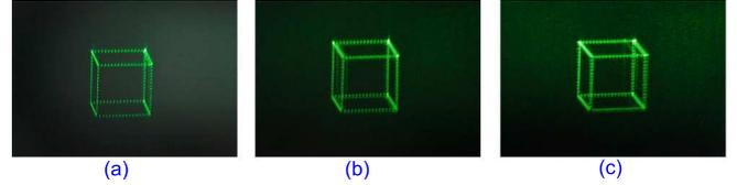
**Fig. 8.** Optical reconstruction of 3D wire-frame model of a cube. (a) Left, (b) center, and (c) right views.
