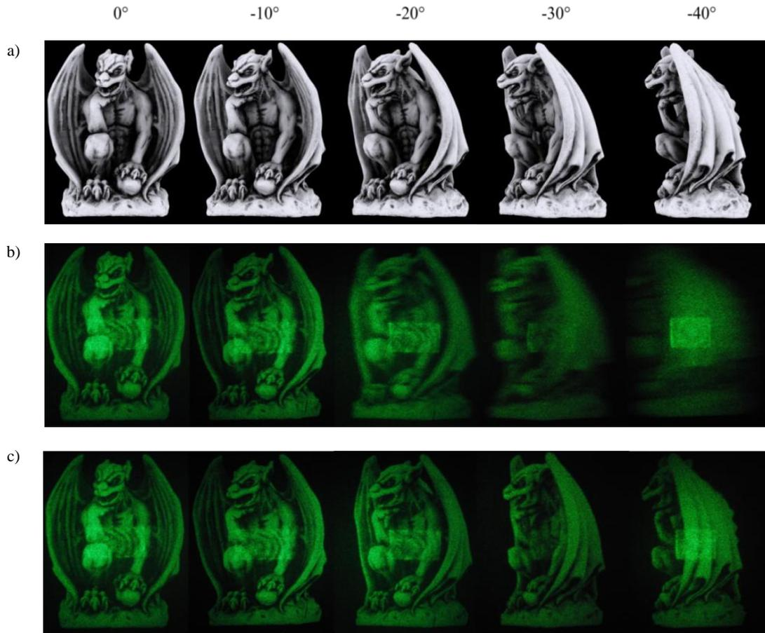
Fig.10: Object (a) and its reconstruction for an inclined illumination without (b) and with tilted planes algorithm use (c) for a tilt angles  $\alpha = 0, 10, 20, 30, 40^\circ$  registered on symmetrically diffusing screen
