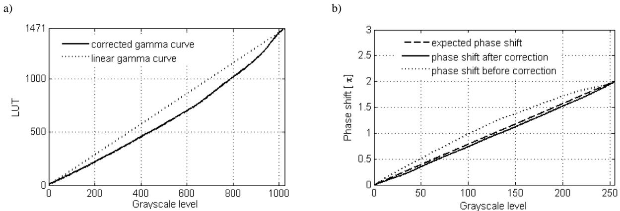
Fig.4 Gamma curves (a) and obtained phase shift characteristics (b) for example LCoS SLM
