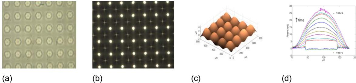
**Fig. 1:** Optical microscope images of the oil coated sample (a) before lens effect start and (b) after complete lens formation; (c) unwrapped phase distribution and (d) Experimental and fitted 1D profiles of the unwrapped phase distribution corresponding to the cooling process;
